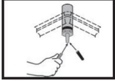
The **DS-2800** is supplied with an overflow protection tube to be installed in the hole of the pan. Although we strongly recommend using it, if you don't want to take advantage of the overflow feature or if you don't have a floor drain, leave the factory installed vinyl cap on the spigot.
