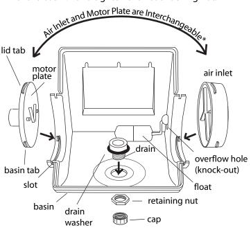
\*interchangeable: install air inlet on the side closest to the hot air supply take-off.
